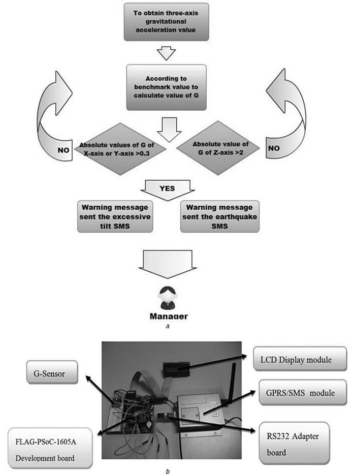
Fig. 4 Bridge inclination monitoring system
