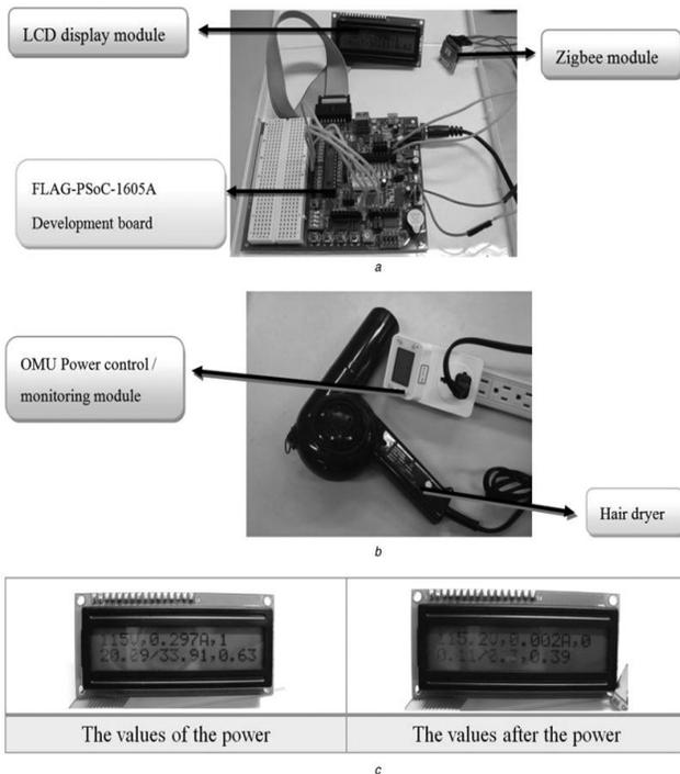
Fig. 6 Smart grid monitoring system
